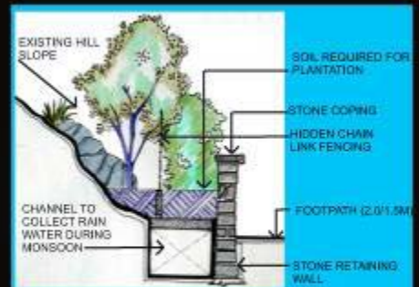
SECTION THROUGH BOUNDARY WALL NEAR MAIN ENTRY
